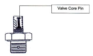
Never exceed pressure rating of the valve. This valve is rated for 2,000 PSI. All component parts used in the system to charge the valve must also be rated to be able to withstand the rated pressure or working pressure of the valve.
