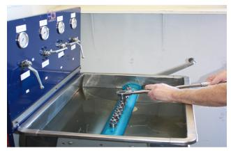
Valves are tested in submersion tanks at their operating pressure to ensure product reliability and trouble-free performance
