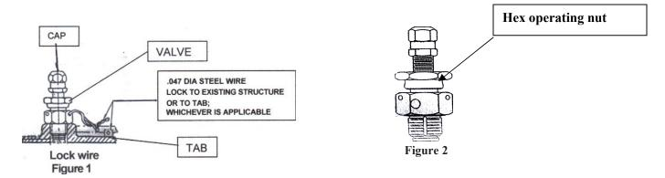
Never exceed pressure rating of the valve. This valve is rated for 5,000 PSI. All component parts used in the system to charge the valve must also be rated to be able to withstand the rated pressure or working pressure of the valve.
